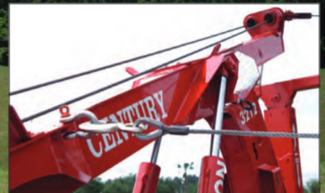
The 3212 G2 allows the cable to be run through a snatch block and hooked to a clevis at the base end of the boom for side pull applications.
